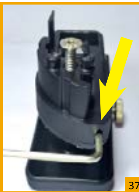
The adjuster screw is at the same height as the box
