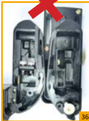
The left side has not been adjusted in accordance with the right side.
